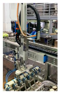
The drive of the manipulator on the basis of the servo drive, which provides an accurate and stable transfer of the wafer production ice cream cup (torch) and sugar cone.
